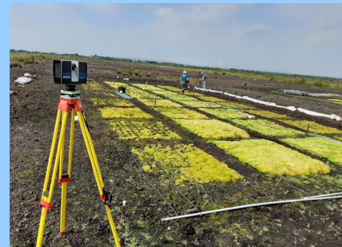
TLS in use at Innovate UK site ©Jack Clough
