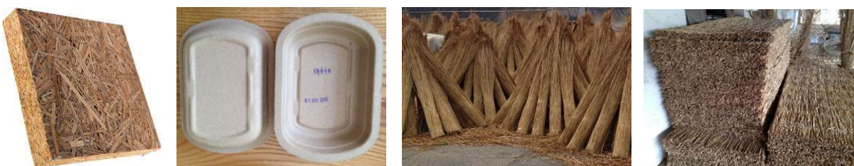
Photos: Products from paludiculture biomass (left: Construction board, molded part, reed bundles for roofing material, right: Insulation boards).
