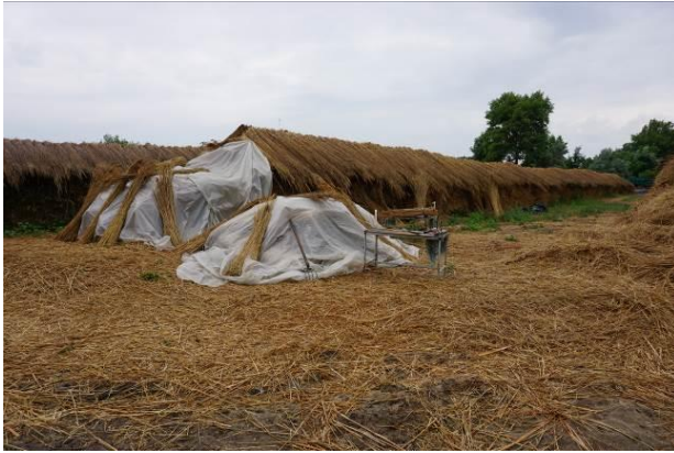
Figures 4 and 5: (l): raw bundles are piled in open-air stacks, in the front, a work bench for manual processing of the raw bundles surrounded by waste reed. (r): bundles, ready for shipping abroad, are piled up for final drying at the open air.
