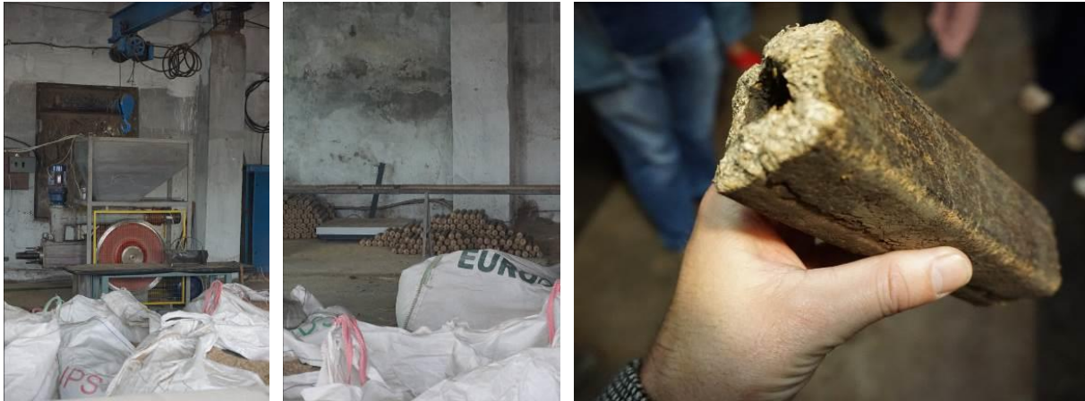
Figures 14, 15, 16: (l & m): Briquetting line for cylindrical reed briquettes of company Dniestroviez; (r): The second type of reed briquette produced by Dniestroviez.
