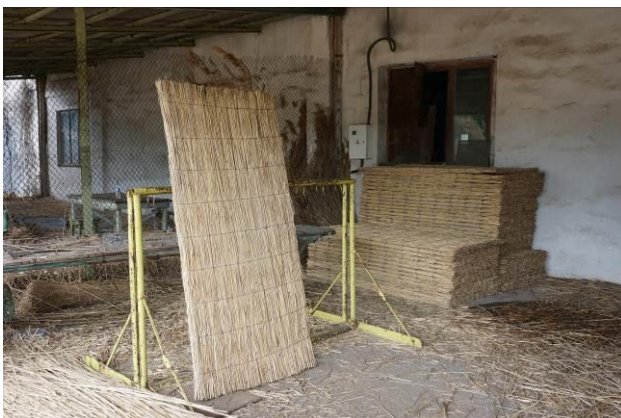
Figures 12 and 13: (l): Manual construction plates production; (r): The CEO Andrey Bulavin of Dnestroviez company during explanations.
