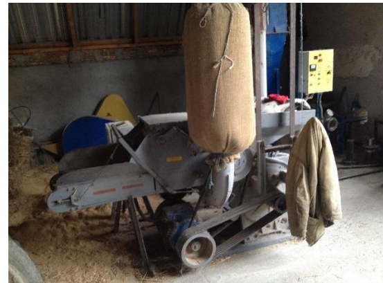
Figures 8 and 9: (l): small reed bales stored for further processing to briquettes, (r): briquetting line with a disintegration unit, hammer mill, and pressblock.
