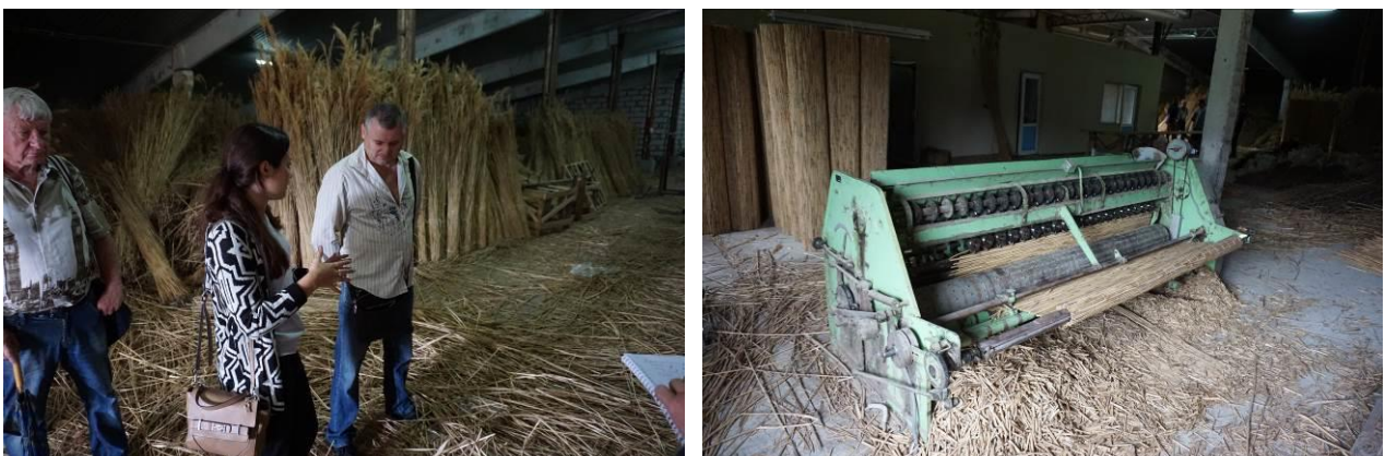
Figures 17 and 18: (l) R. Wanner explaining the focus of LLC “Ecodnestr” on production of reed thatch and mats for export; (r): Halve automatic loom for reed mats.
