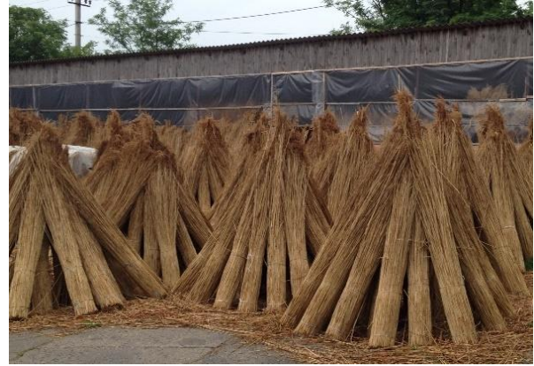
Figures 4 and 5: (l): raw bundles are piled in open-air stacks, in the front, a work bench for manual processing of the raw bundles surrounded by waste reed. (r): bundles, ready for shipping abroad, are piled up for final drying at the open air.
