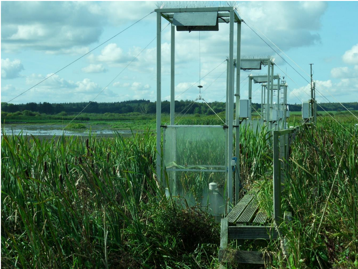
(d) Automatic flux measurement chambers and an eddy covariance system to determine turbulent exchange fluxes of heat, water vapor, CO 2 , and CH 4 between a re-wetted peatland and the atmosphere at Zarnekow, NE Germany. These devices are run by the Helmholtz Centre Potsdam, GFZ German Research Centre for Geosciences (photo taken in September 2016, W. Wichtmann)
