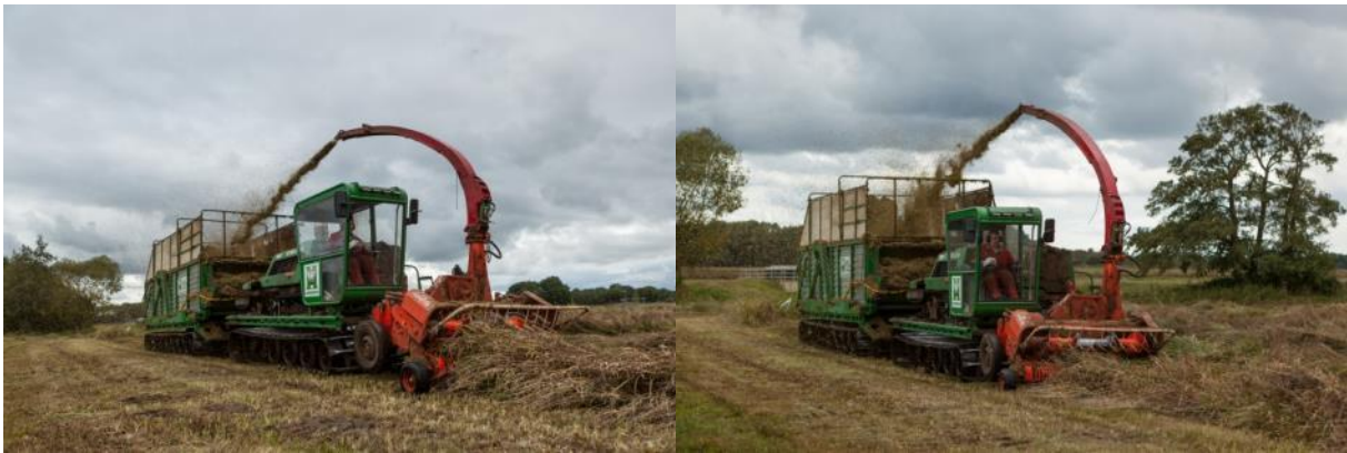
Fig.: Hanze Wetlands new tracked vehicle chopping biomass
